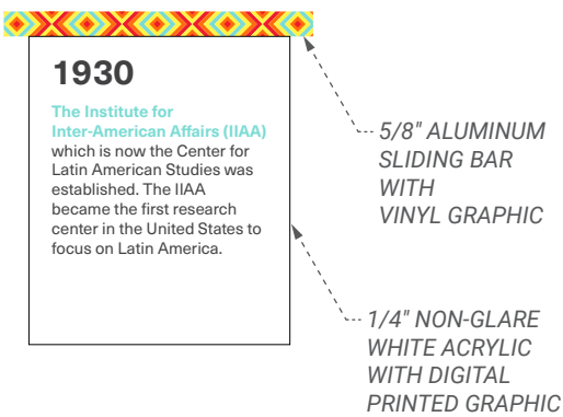
LAYOUT A3 FRONT VIEW DETAIL SCALE: 1 1/2"=1'-0
