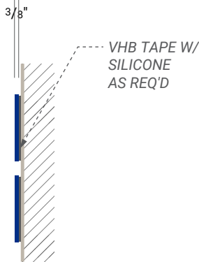
SIDE VIEW DETAIL SCALE: 1"=1'-0
