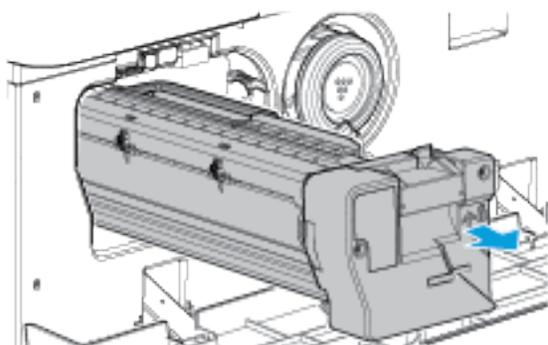
6. Lift the carrying handle on the top of the cartridge and use it to support the weight while you remove the cartridge from the printer.
