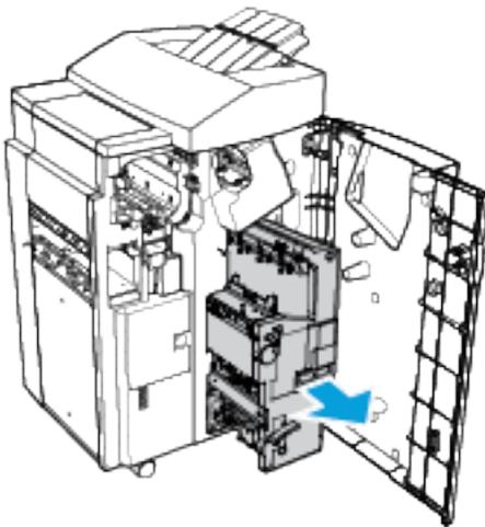
3. To access the staple cartridge unit, pull down the green tab.
