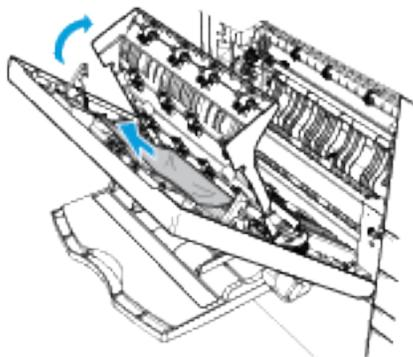
3. Close the left side door, then wait 10 seconds. Any paper currently in transport inside the printer moves to the left side area.
