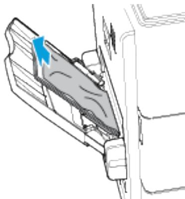
2. Ensure that the paper-feed entrance where the tray connects to the printer is clear.
