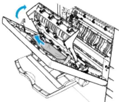
2. Close the left side door, then wait 10 seconds. Any paper currently in transport inside the printer moves to the left side area.
