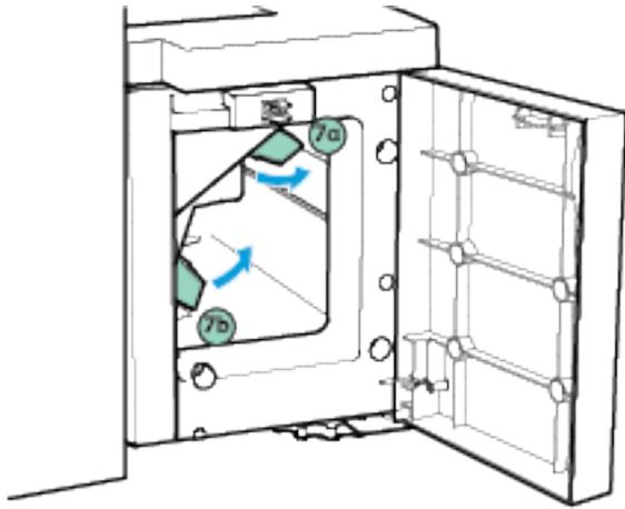
Ensure that you have removed all jammed paper, and that jam area covers are closed correctly.
