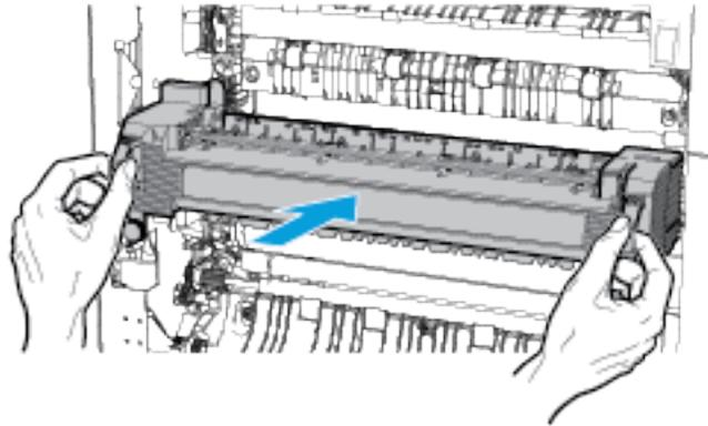
8. To fasten the fuser module, rotate the orange thumbscrews clockwise.
