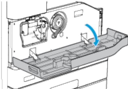
2. Rotate the orange print cartridge locking lever counterclockwise until it clicks. The lever is to the right of the print cartridge unit.
