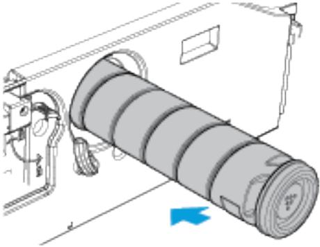
6. To lock the toner cartridge into place, rotate the orange toner cartridge locking lever clockwise.
