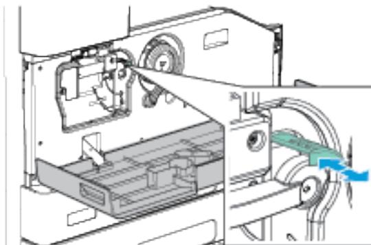
4. To clean the printhead, push the blue handle gently back into the printer.
