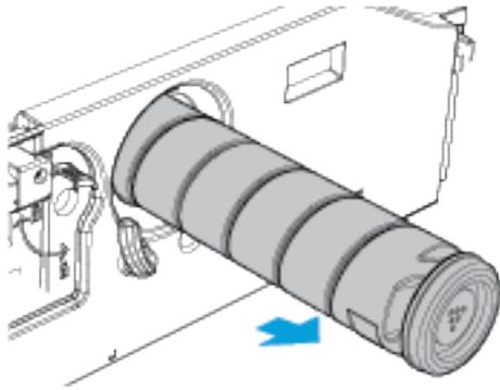
4. Remove the new toner cartridge from the packaging. Tilt the cartridge up and down, then left and right 10 times.
