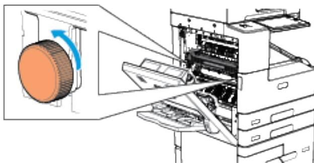
5. Pull out the used fuser module.
