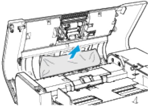
3. If the original document is not visible when the top cover is opened, lift the document feeder.
