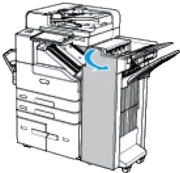
2. Slide the hole-punch waste container out of the finisher.
