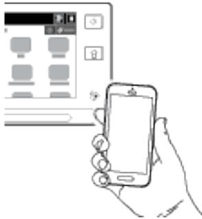
The mobile device and the printer communicate with each other. The mobile device searches the network for the printer. When the printer is located, it is added to the list as a mapped printer.
