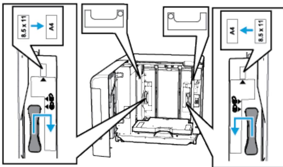
3. To secure the paper guide, slide down the paper-guide retainer to the lock position.
