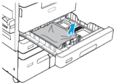
6. If the paper is torn, remove the tray completely, then check inside the printer for torn pieces of paper.
