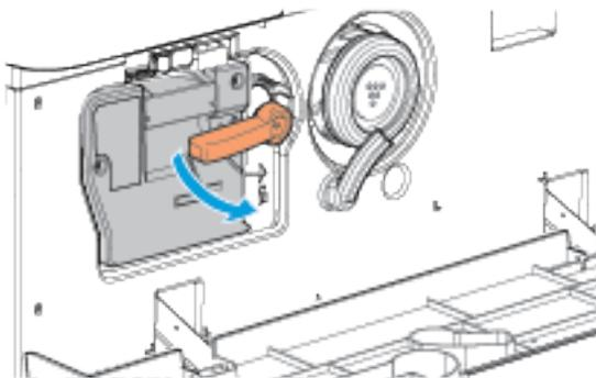
3. Locate the blue handle at the top right of the print cartridge. Pull out the print cartridge about 40 cm or 16 in., until it stops.
