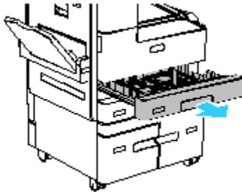
2. To expand the length or width paper guide, release the guide lock, then slide out the length or width paper guide until it stops.
