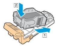
8. Grasp the staple cartridge by the orange handle, then insert it into the stapler assembly. Push the staple cartridge in until it clicks.
