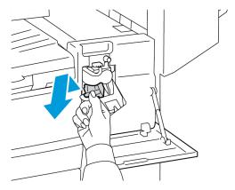
5. Pinch both sides of the staple pack and remove the staple pack from the cartridge.
