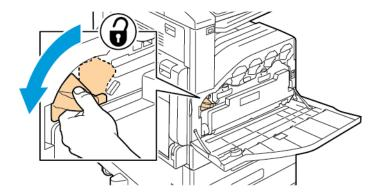
b. To release the waste cartridge, press the orange tabs as shown.
