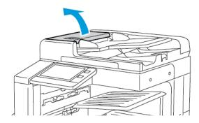
2. If the original document is clear of the automatic document feeder entry, pull it straight out in the direction shown.
