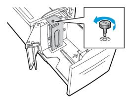
2. To remove the spacer plate, grasp the spacer plate and lift upward.
