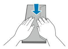
3. Load Number 10, C5, DL, or Monarch envelopes with flaps facing up and the long edge going into the printer first.
