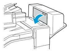
2. If the staple cartridges are not visible, grasp the vertical panels on each side of the opening, then slide the staple cartridges to the center.
