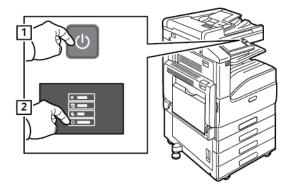
b. Open the front door, then press the power switch off.
