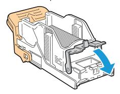
9. Grip the staple cartridge by the orange handle and insert it into the stapler assembly. Push it in until it clicks.
