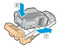
7. Grasp the new staple cartridge by the orange handle, then insert the cartridge into the stapler assembly until it clicks.
