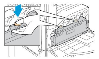
c. Grasp the handle of the waste cartridge, then pull it out.
