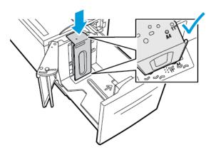
5. Install the screw to secure the spacer plate.
