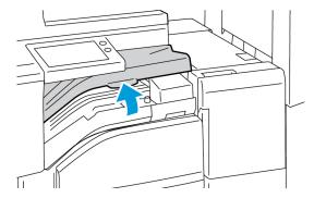
2. Pull out the hole-punch waste container.
