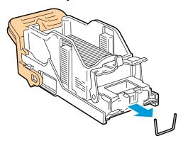
8. Push the clamp in the direction shown until it snaps into the locked position.
