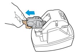
3. Unpack the new staple cartridge. Remove any partial strips and any staple strips that are not flat.
