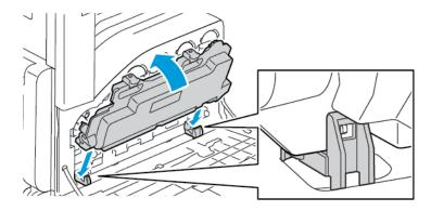
b. Press the waste cartridge toward the printer, until it clicks into place.
