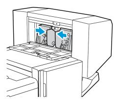
3. Hold the tabs on both sides of the staple cartridge and pull the cartridge out of the finisher.
