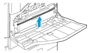
4. Slowly push the cleaning rod into the printer until it stops, then pull it out. Repeat this action two more times.
