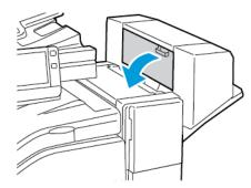
2. If the staple cartridges are not visible, grasp the vertical panels on each side of the opening and slide the staple cartridges to the center.
