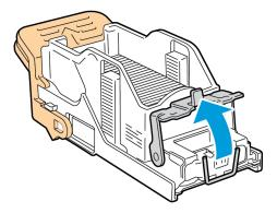
7. Remove the jammed staples, then push the clamp in the direction shown until the clamp clicks into the locked position.
