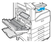
4. If paper is jammed in the Fuser, remove the paper from areas A1 and A2 as shown.
