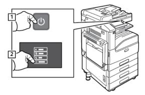
2. Open the front door, then press the power switch off.
