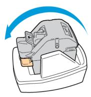
2. Grip the staple cartridge and pull it out of the stapler head.
