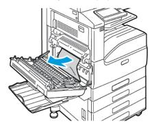
3. If paper is jammed at the exit to the output tray, to remove it, carefully pull it straight out in the direction shown.
