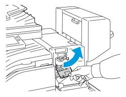
4. To remove the staple cartridge, grasp the orange handle, then pull it firmly toward you.
