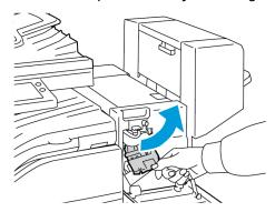
4. To remove the staple cartridge, grasp the orange handle, then pull the handle toward you.
