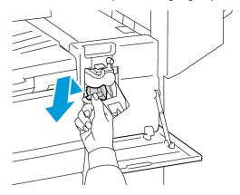
5. Check inside the finisher for any loose staples, then remove the staples.
