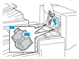
4. To remove the jammed staples, pull the staples in the direction shown.
