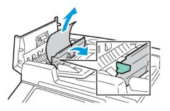
4. To remove the original document from the feeder, rotate the green wheel in the direction shown, then carefully pull out the document.
