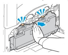
c. To lock the waste cartridge, rotate the waste cartridge lock lever 90 degrees clockwise.
