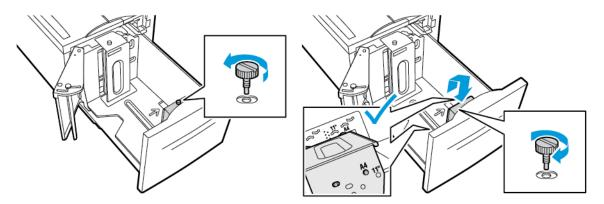
7. On the top of the side gate, locate the pin.
