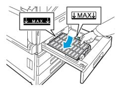
• For short-edge feed, insert labels face up with the top edge to the left
