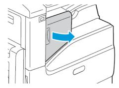
2. To remove the staple cartridge, grasp the orange handle, then pull it firmly toward you.
