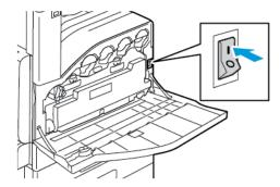
2. At the printer control panel, press the **Power/Wake** button.
