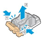
7. Insert the front side of the new staple pack into the staple cartridge, then push the rear side into the cartridge.
