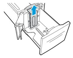
3. Place the tabs at the bottom of the spacer plate into the slots in the bottom of Tray 6 that correspond with the paper size.
