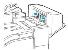
3. Hold the tabs on both sides of the staple cartridge, then pull the cartridge out of the finisher.
