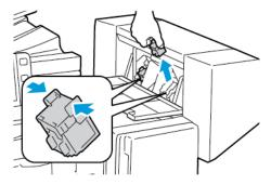
4. Remove the new stapler cartridge from its packaging. Hold the tabs on both sides of the new staple cartridge, then reinsert the staple cartridge into the original position in the finisher.
