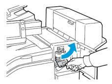
4. To remove the staple cartridge, grasp the orange handle, then pull it firmly toward you.
