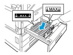
Note: Do not load paper above the maximum fill line. Overfilling the tray can cause paper jams.
