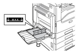
• For short-edge feed, load labels face down with the top edge to the right.
