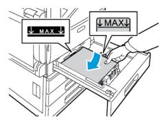
6. To adjust the length and width guides to fit the paper, pinch the guide locks, then slide the paper guides in until they touch the paper.
