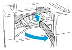
2. Pull out the hole-punch waste container.
