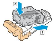
6. Grasp the new staple cartridge by the orange handle, then insert the cartridge into the stapler until it clicks.
