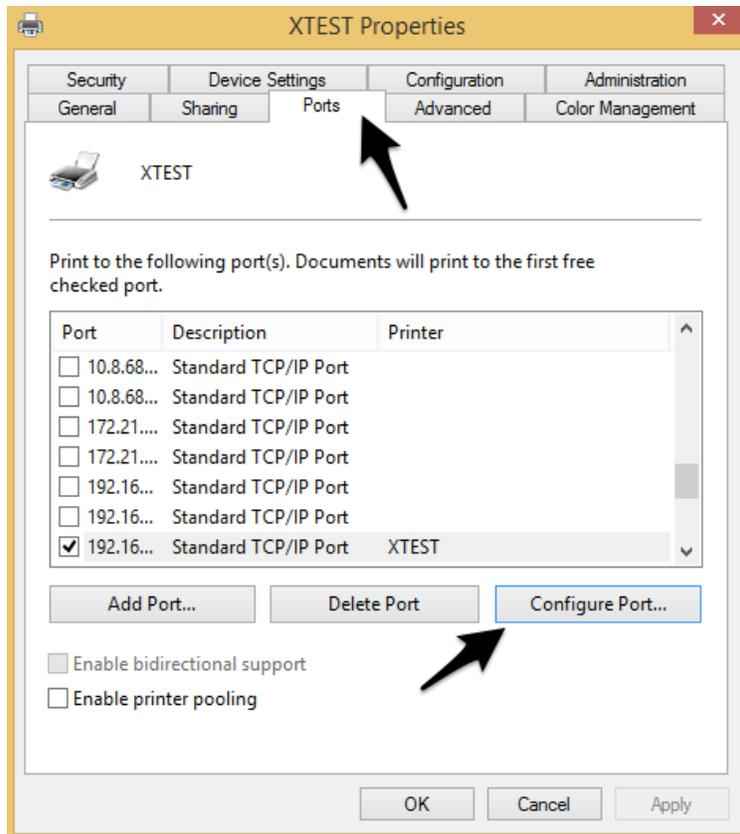
**Change the Protocol from RAW to LPR, set the Queue Name to 'lp' (lowercase LP), and uncheck both LPR Byte Counting and SNMP Status, if either one are checked (in some cases both may be checked or one or the other). Click OK.**
