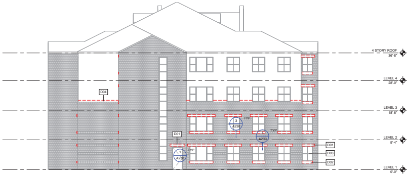
3 DEMO ELEVATION - 4 STORY BUILDING - SIDE (TYPICAL) 1/8" = 1'-0"
