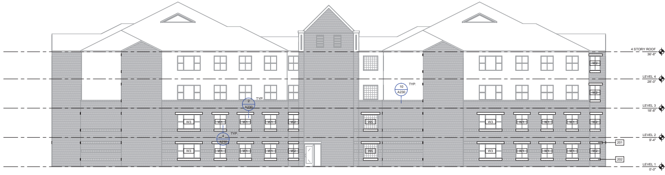
2 NEW WORK ELEVATION - 4 STORY BUILDING - BACK 1/8" = 1'-0"
