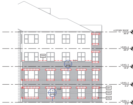
4 DEMO ELEVATION - 4 STORY BUILDING - STAIR ADJACENT (TYPICAL) 1/8" = 1'-0"
