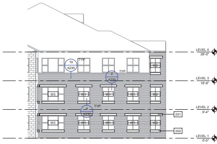
4 NEW WORK ELEVATION - 3 STORY BUILDING - STAIR ADJACENT (TYPICAL) 1/8" = 1'-0"
