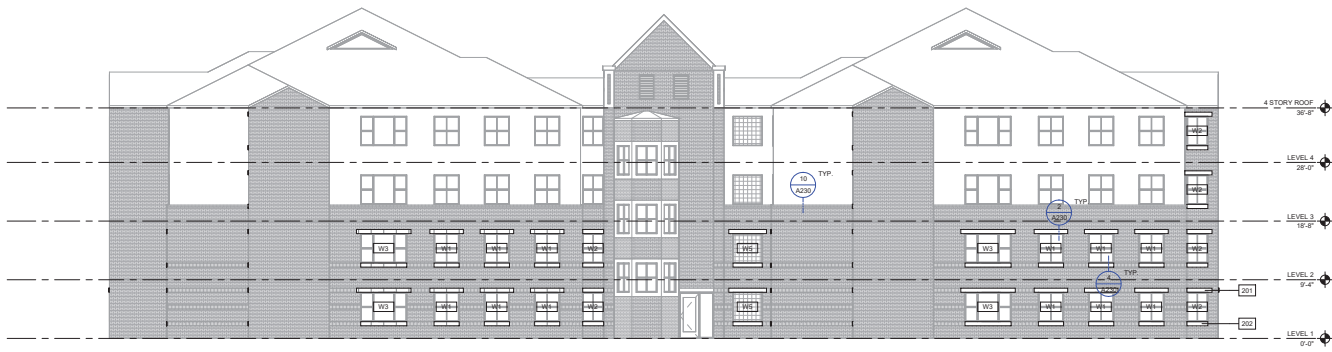
1 NEW WORK ELEVATION - 4 STORY BUILDING - FRONT 1/8" = 1'-0"
